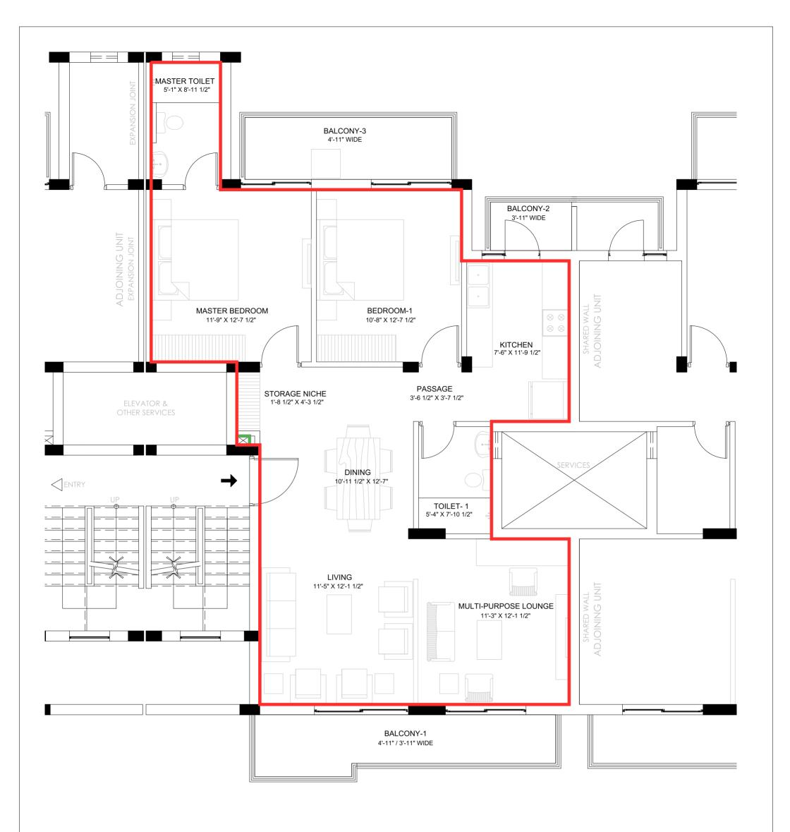
\* APPROX. INTERNAL DIMENSIONS CLEAR OF MASONRYWORK,LOSS OF 2.5-4.0 CM IS EXPECTED ON ACCOUNT OF PLASTER, SKIRTING & OTHER FINISHES.
