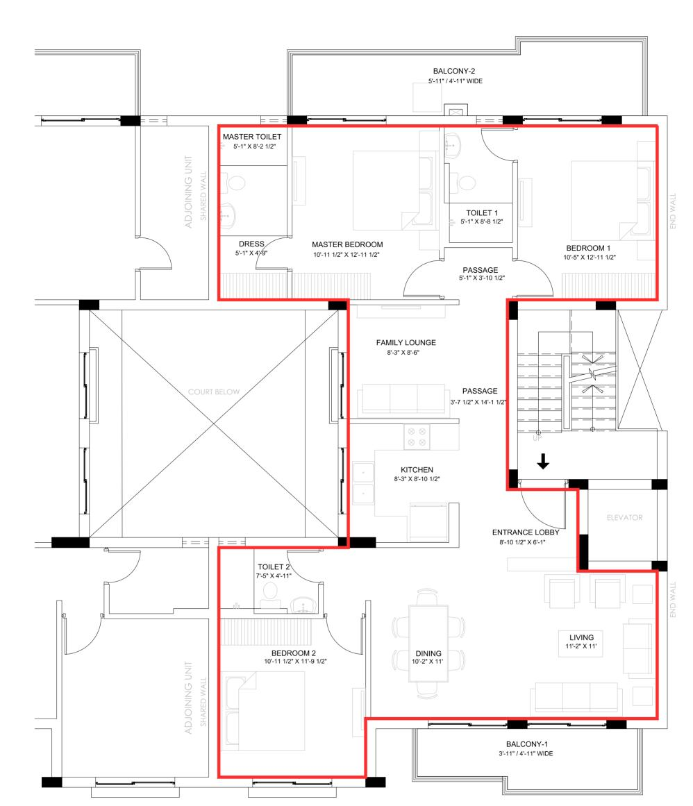
\* APPROX. INTERNAL DIMENSIONS CLEAR OF MASONRYWORK,LOSS OF 2.5-4.0 CM IS EXPECTED ON ACCOUNT OF PLASTER, SKIRTING & OTHER FINISHES.
