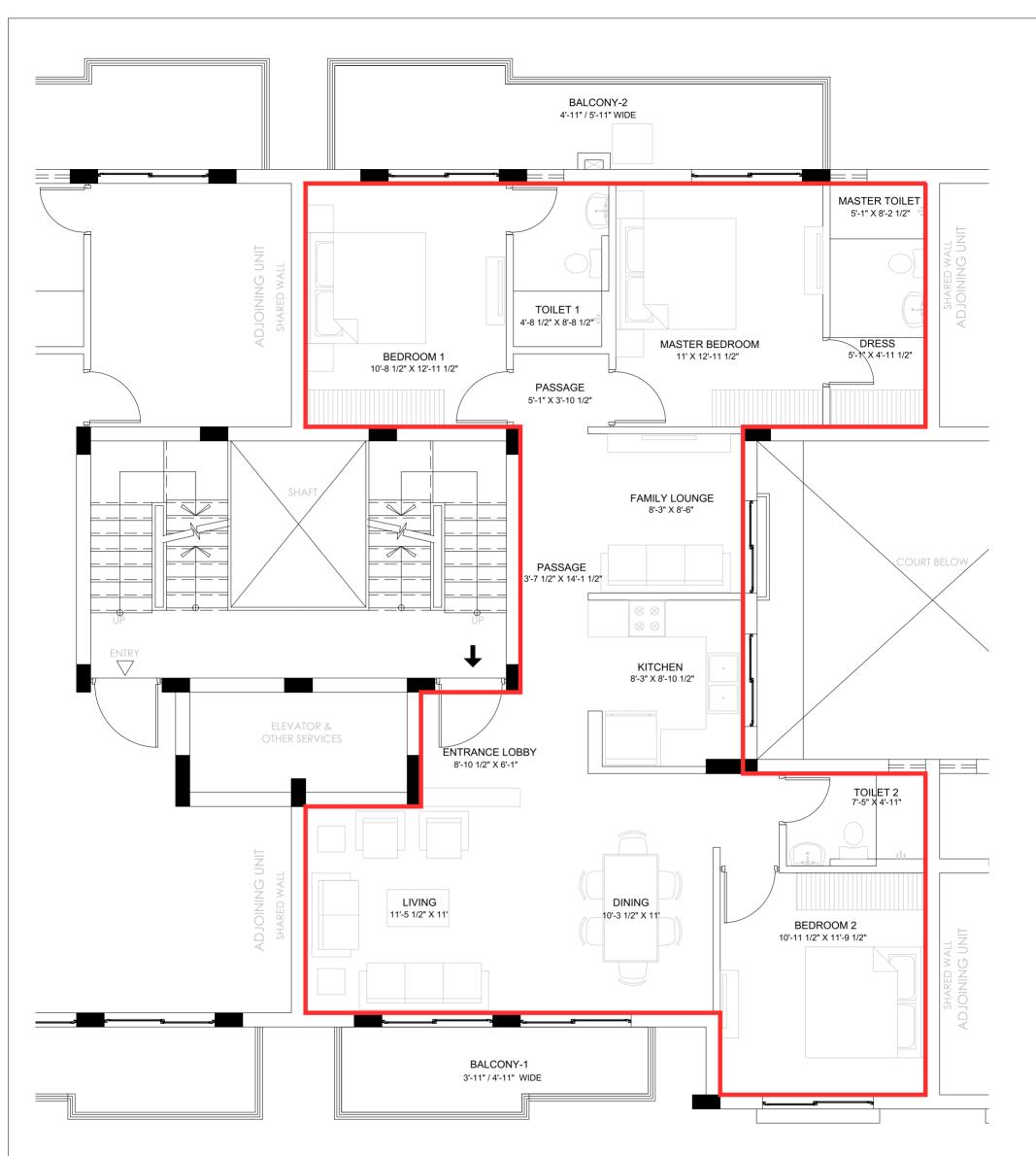
\* APPROX. INTERNAL DIMENSIONS CLEAR OF MASONRYWORK,LOSS OF 2.5-4.0 CM IS EXPECTED ON ACCOUNT OF PLASTER, SKIRTING & OTHER FINISHES.
